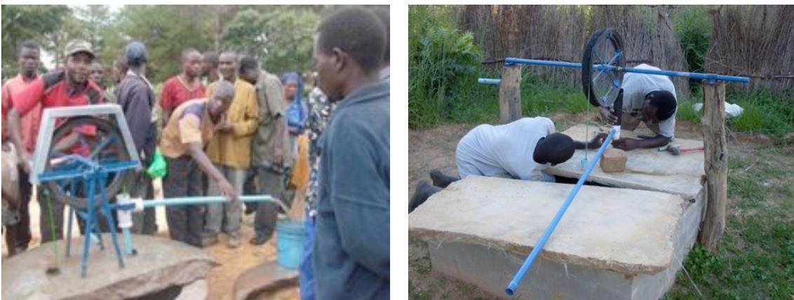
Figure 8: Pictures show two types of pumps used in the project – Left, the A model and right, the pole model. The project set up both types for demonstration with the model farmers.
