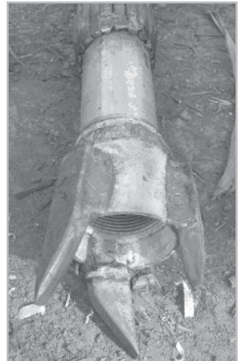
*Teeth of drill bit from steel from truck springs*
