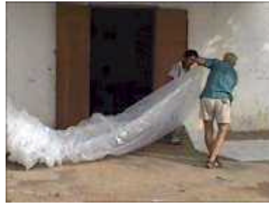
Photo 3. Putting one plastic inside the other to give added strength
