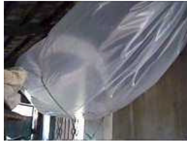
Photo 17. A string around the bag is used to increase the pressure
