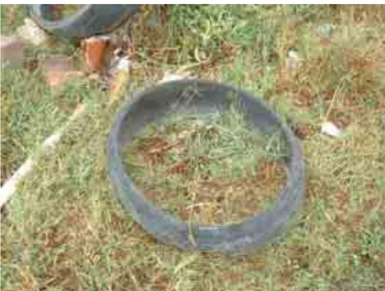
The rubber circles are cut out from a car tyre by cutting along the part of the tyre which normally touches the road.
